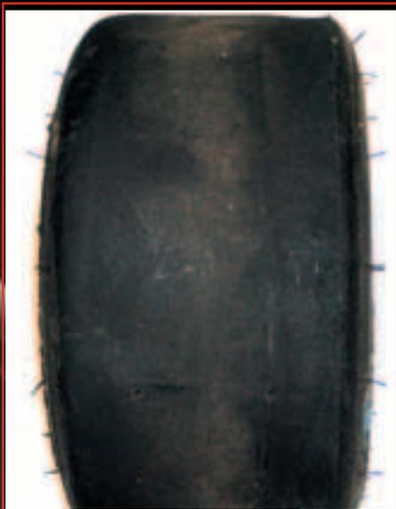
The air pressure in this tire was too low. The tire surface is very contorted and the outside edges show the effects of too much sidewall flex, thus the shredding of the outer edge.
